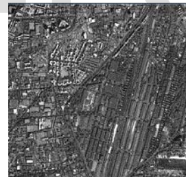
FIG H: OUTPUT OBTAINED BY APPLYING LAPLACIAN OPERATOR
